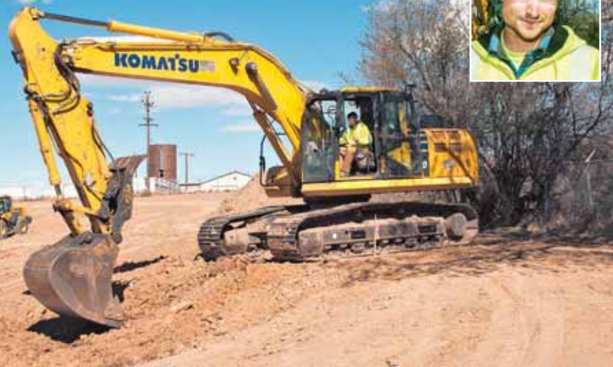
Operator Brandon Allen digs with a Komatsu PC210LC-10 excavator on a jobsite in Greeley.
