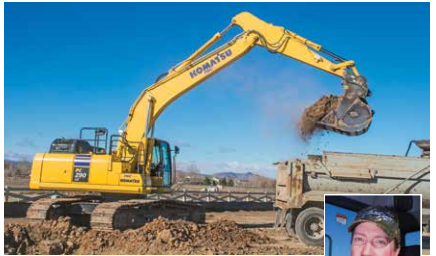
Project Foreman Ryan Selander digs and loads a truck with a Komatsu PC290LC excavator on a residential project. “It has good power and reach,” said Selander. “I’m digging more than 10 feet deep, coming up out of hole to dump in the trucks, and it helps that it has good speed through the entire cycle. It has increased production.”
